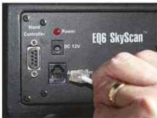
▲ Attach the ST-4 cable from the guide camera to the port on your mount
